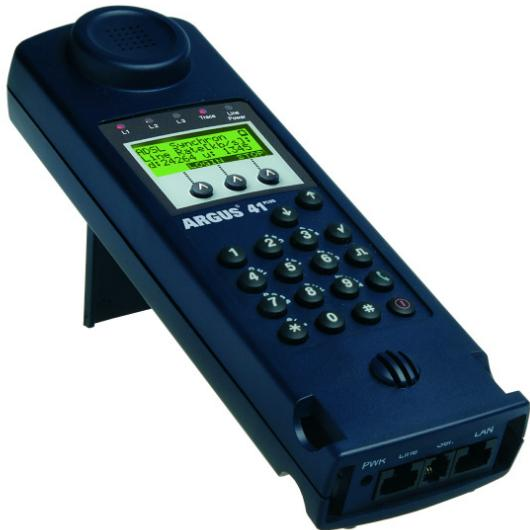
ARGUS® 41PLUS allows the installer to confirm that the promised ADSL service is being properly delivered to the subscriber.
